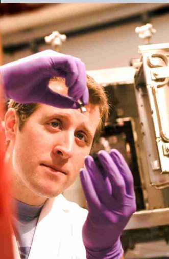
Nikolas Hrabe prepares a sample of porous titanium for heat treatment in a high vacuum furnace.
